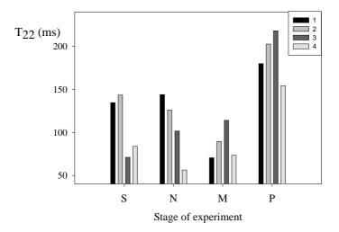
**Fig. 3.** Changes in the value of the long component  $T_{22}$  value for individual phases of the experiment: (S – untreated muscle, N – muscle injected with brine, M – massaged muscle, P – pasteurized muscle), (1 – pork musculus longissimus dorsi, 2 – pork musculus semimembranosus, 3 – beef musculus longissimus dorsi and 4 - beef musculus semimembranosus)
